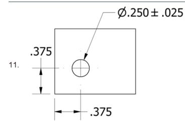
The front view of a part is shown above. What is the tolerance on the hole diameter?
