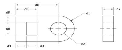
What would be the parametric equation for dimension d7 if the depth of the part is always to be 1/4 of d0?
