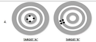
Accuracy is defined as "The ability of a measurement to match the actual value of the quantity being measured." Precision is defined as "The ability of a measurement to be consistently reproduced". The images each show four attempts to approximate the center of the target, illustrating the concept of accuracy and precision. Based on the images, select the correct statement about precision and accuracy.
