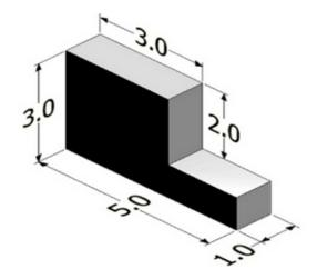
The multi-view drawing details an aluminum part and shows dimensions in centimeters. A rubber coating will be applied to the outside surface of the part such that 1 liter covers 2000 square centimeters.
