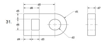
What is the parametric equation for dimension d2 if the diameter of the hole is always to be 1/3 of d0?
