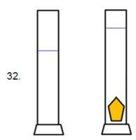
An irregularly shaped object has a mass of 150 grams. You have a graduated cylinder that contains 100 mL of water and when the object is placed into the cylinder the volume of water increases to 140 mL. What is the density of the material of the object?
