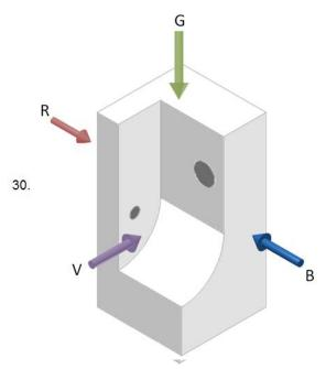
Use the randomly oriented pictorial view of the object to answer the question. Which line of sight (indicated by arrows) is the <u>BEST</u> choice to use in order to create the **front** view orthographic projection?
