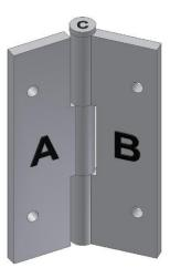
10.4: How many degrees of freedom are left once the parts of the hinge are assembled?
